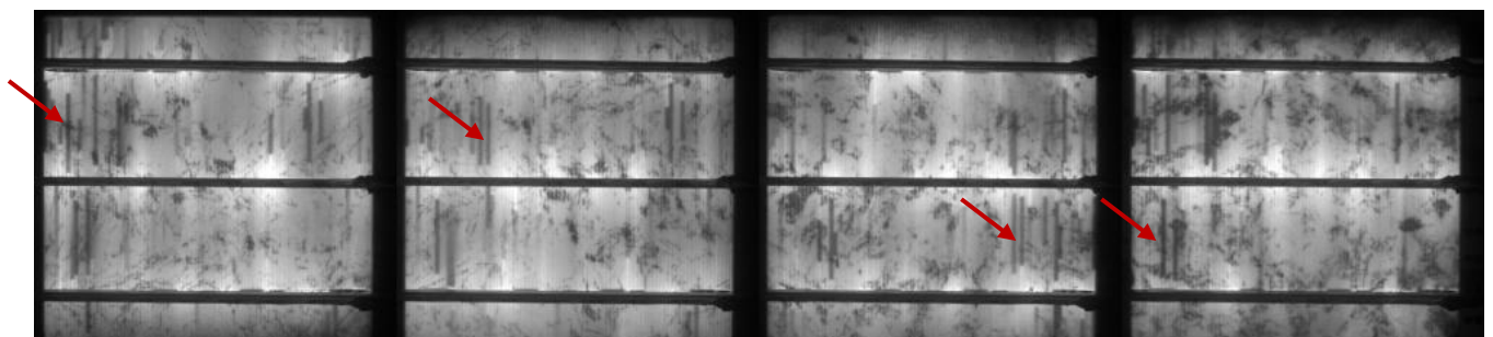
Figure 7 – Breaks in the silver screen print grid on the front show up as black lines running perpendicular to the busbar in the EL image.
